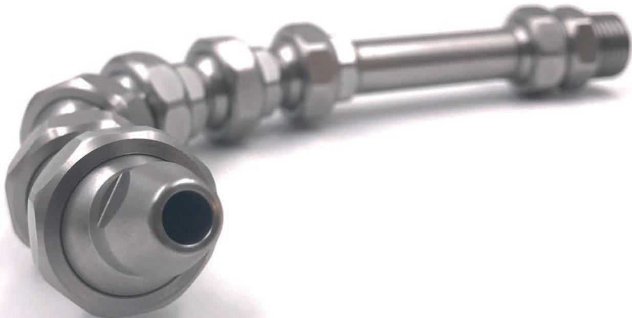
The Type 1 system for all machine applications in the range up to  $\pm 170\text{l/min}$ . With round nozzles sizes from  $\varnothing 1.6\text{ mm}$  to  $\varnothing 5.0\text{ mm}$  and a variety of flat nozzles and multi-bore nozzles, this system is a standard for every machine. The wide range of machine adapters from M8x1.0, M14x1.5 and G3/8" to various ball adapters with  $\varnothing 14.0\text{ mm}$  and of course also basic and angled elements guarantee a smooth installation.
